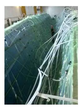
With Sicomin's support, H2X ran numerous tests to ensure they had the precise viscosity levels and gel times to ensure the SR8100 resin flowed through the reinforcements quickly without leaving dry spots. "You don't want a gel time so long that there is too much time between completion of wet out and beginning of gel", Pierre Lallemand of H2X remarks. "This wastes time and money and increases risk."
