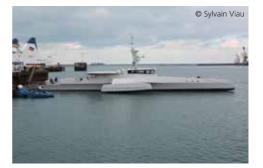
The first fully assembled boat took 3 months in total to complete and Sicomin and H2X's overall attention to process control and material selection paid dividends. "The weights of the first and second boats' main hulls differed by less than 5kg – impressive for such a large structure," comments Lallemand of H2X.
